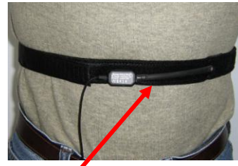
The rubber strap stretches when the abdomen expands during breathing.
